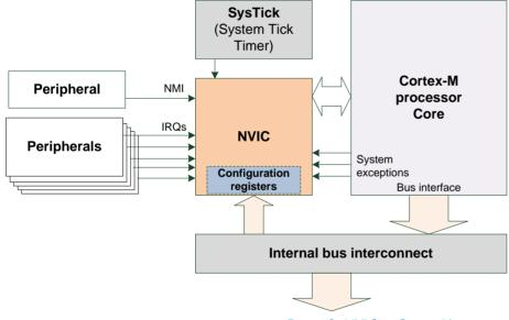
Figure 2: NVIC in Cortex-M processor
