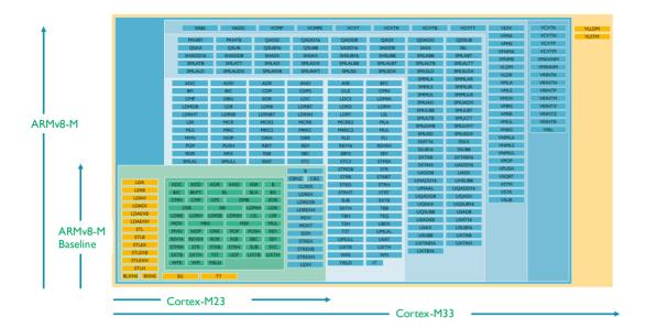
Figure 3: Instruction Set support in the Cortex-M processors
