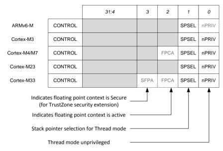
Figure 6: The CONTROL register
