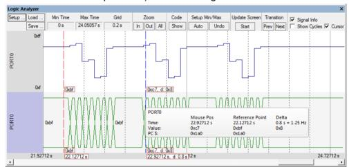
Figure 13: Logic Analyzer in Keil μVision debugger
