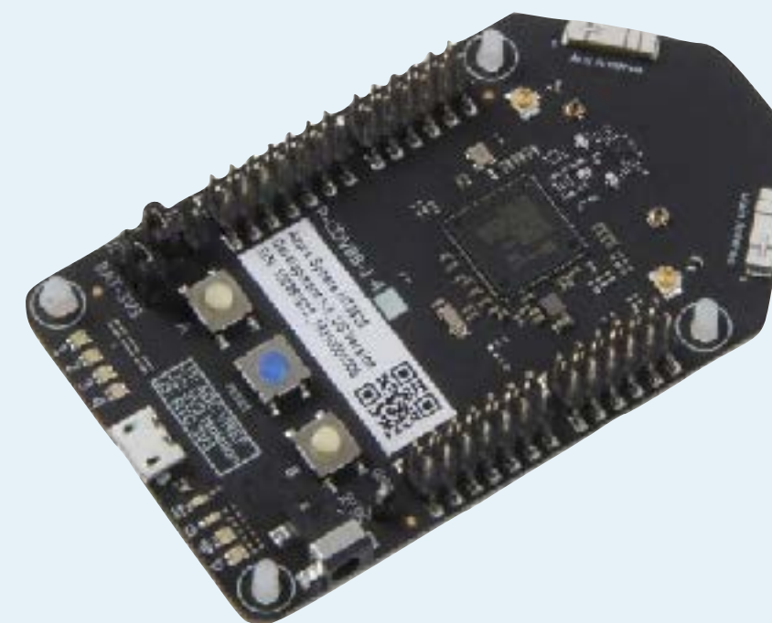
AzureSphere: Microsoft's secure edge IoT device
