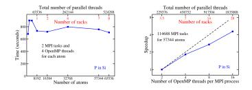
(left) weak-scaling obtained by increasing the number of MPI tasks together with the number of atoms, (right) scaling to the full machine by increasing the number of OpenMP threads while keeping the number of MPI tasks fixed. Both use 64 hardware threads on each node. (Taken from KKRnano High-Q results)
