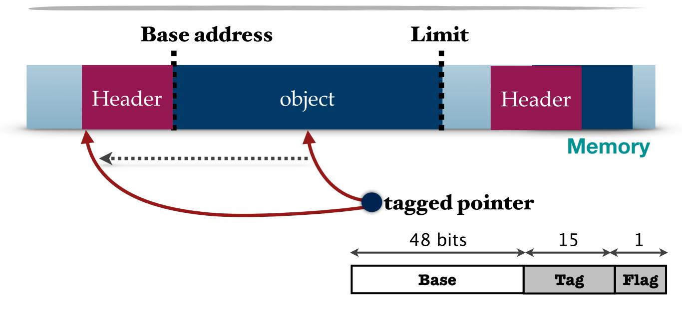
The address of a header is derived from a tagged pointer.
