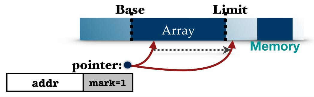
2. Mark out-of-bound pointer at pointer arithmetic.
