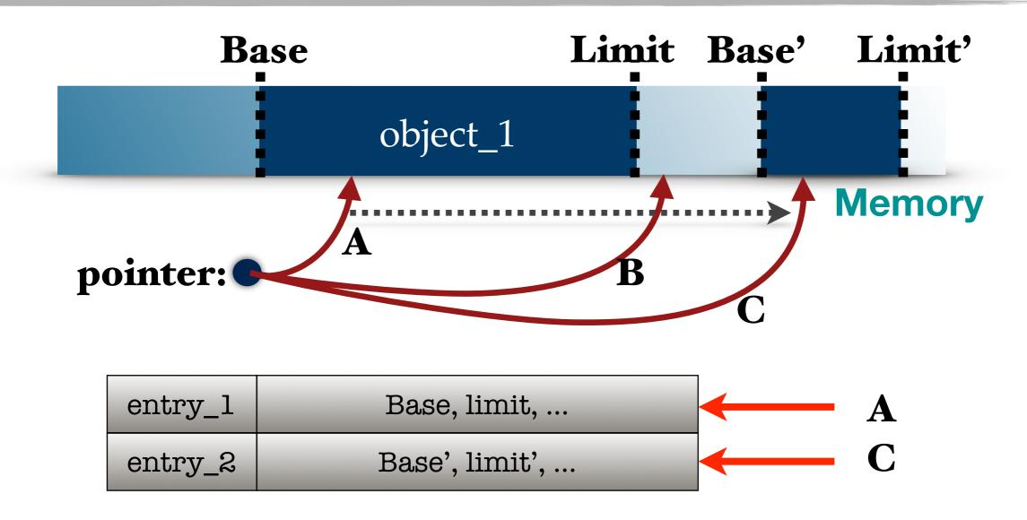
Tracking objects requires checks at pointer arithmetic to keep track of intended referents.
