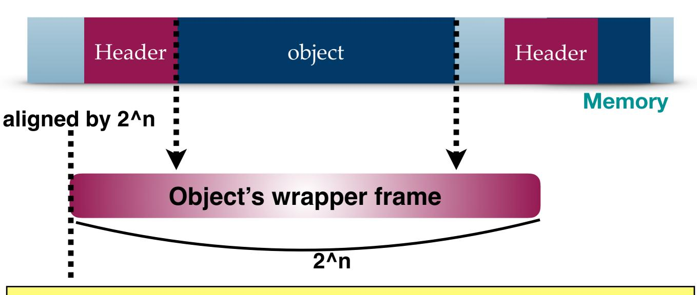
An object's wrapper frame is defined as the smallest frame.
