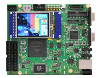
Figure 8 – Cortex-M Prototyping System, an FPGA designed for Cortex-M system development
