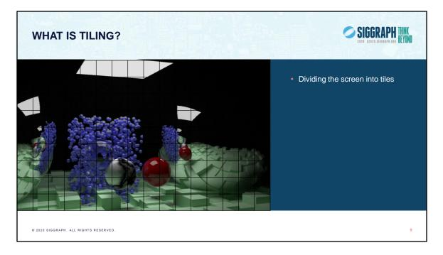
When we talk about a tile-based rendering GPU, this is what we mean. Each render target is divided into a rectangular grid of tiles.
