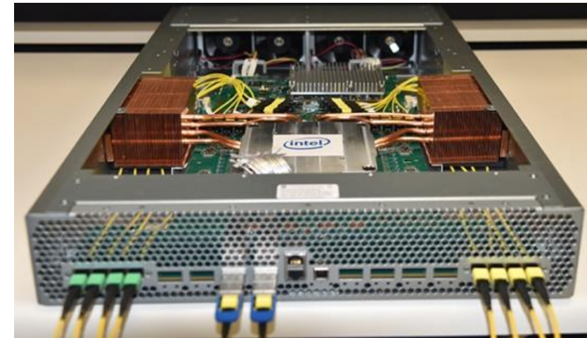
Intel Co-packaged 12.8 Tb/s Switch (2020) SiPh engine @ 1.6 Tb/s
