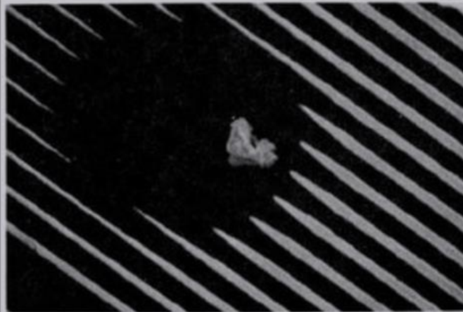
Figure 2: Example of a break of 7 metal lines caused by the interaction between a contaminating particle and the photoresist.
