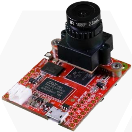
OpenMV CAM Running MicroPython over STM32
