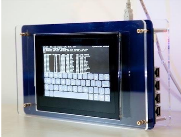
An early experimental FPGA-based CHERI tablet prototype running the CheriBSD operating system and applications, Cambridge, 2013
