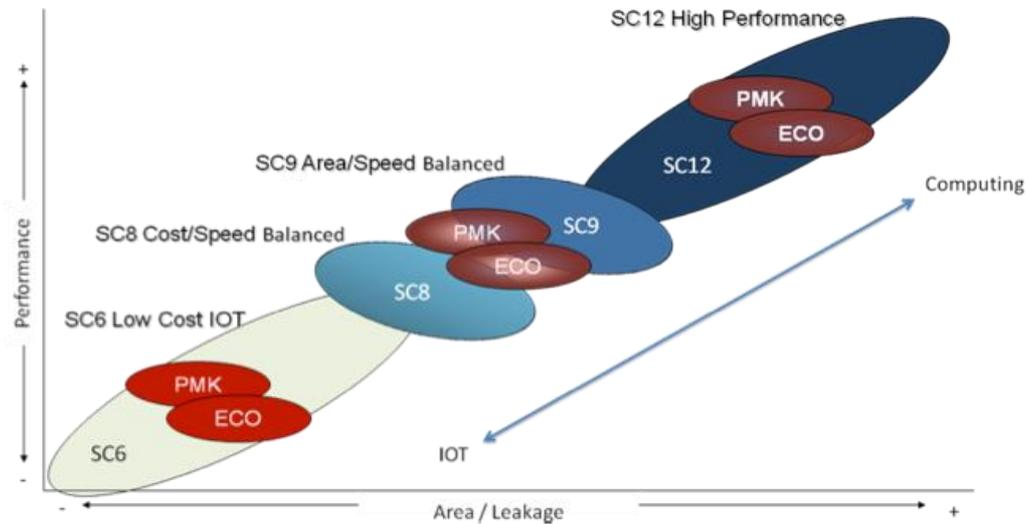
Figure 5 – A wide range of logic cell libraries can be available in a single process node
