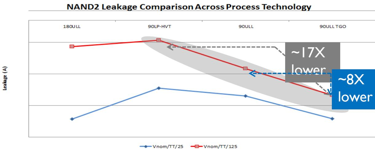
Figure 7 – TGO device provides significantly lower leakage than standard device
