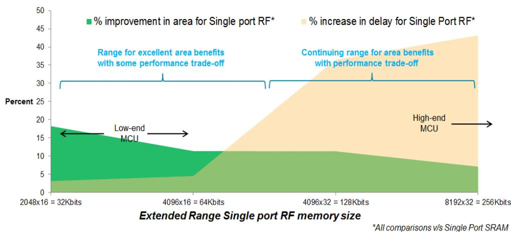
Figure 2 – Single port Register File provides high density memory
