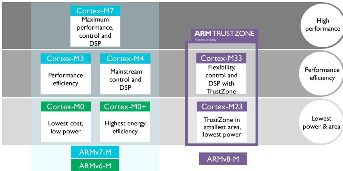
Figure 9 - the ARM Cortex-M processor family
