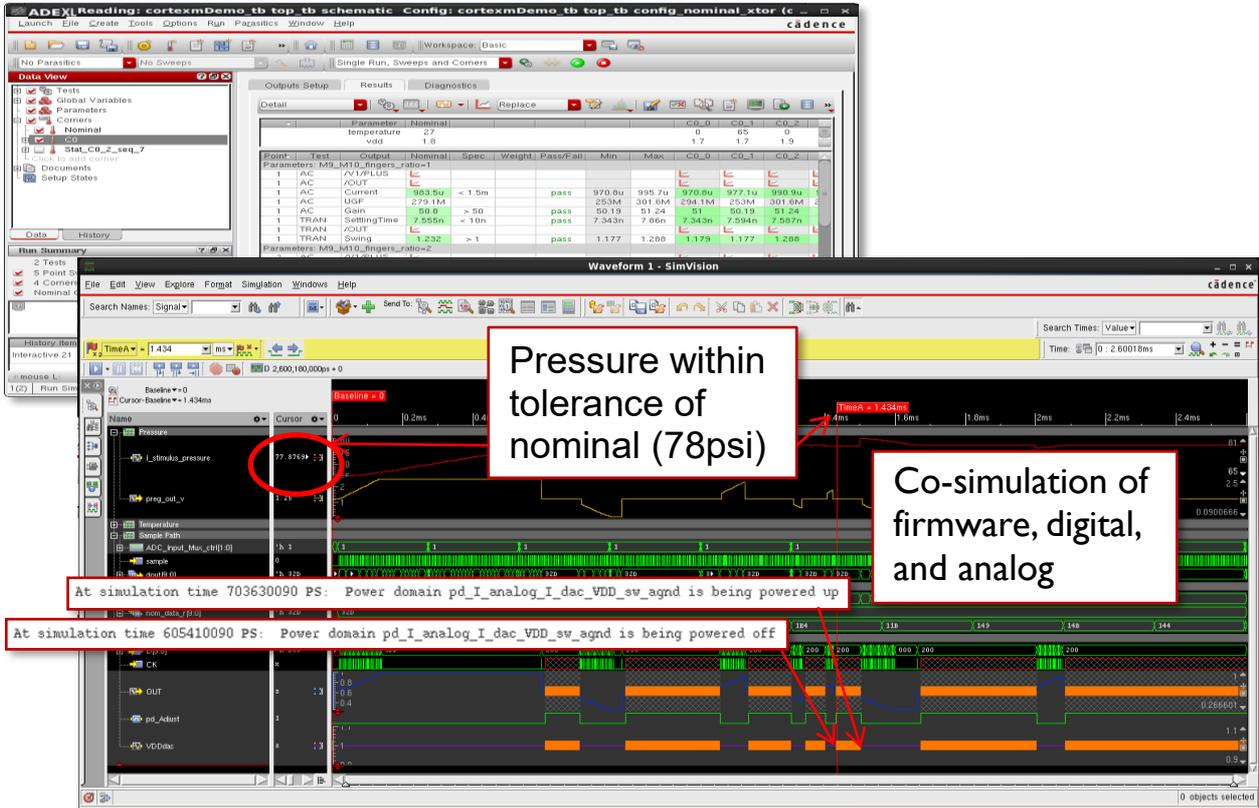
Figure 4 – System Simulation: Virtuoso Analog Design Environment + SimVision
