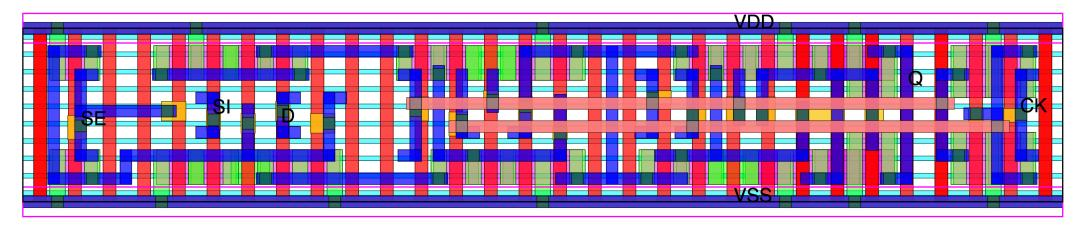
Resize the SDFFQ\_X1N with one-fin transistor
