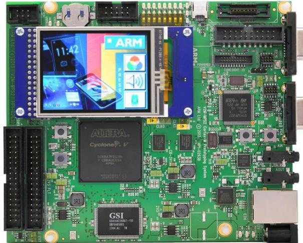
*Figure 8 – Cortex-M Prototyping System, an FPGA designed for Cortex-M system development*
