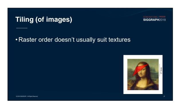
The order in which the pixels in a triangle are processed are unlikely, if the triangle has arbitrary orientation, to suit a simple linear image layout.
