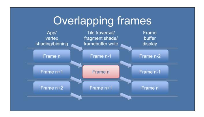
At the end of each frame, the frame buffer is pointed at the most recent rendering result, the rendering pass collects a new set of binned geometry to work on, and the application moves on to the next workload.
