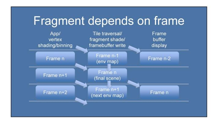
Again, "frames" here refer to the output of fragment shading, not necessarily something for final display.
