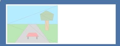
Then each tile is processed (conceptually) in turn, looking at the triangles that are listed as intersecting the tile.
