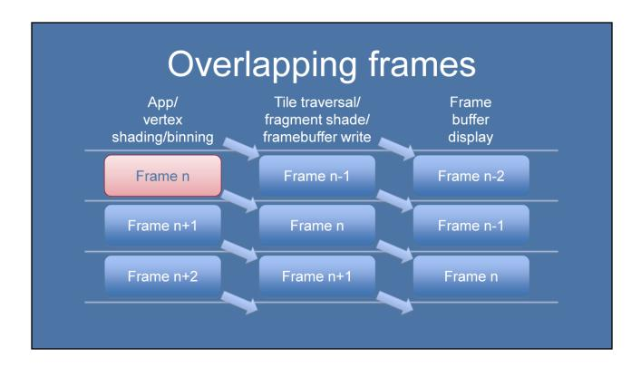
When the rendering pipeline is running efficiently, the application will be submitting geometry, which will be vertex shaded and classified into bins.
