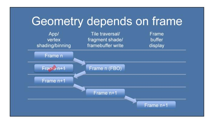
Here we've got frame n+1 being submitted by the application, but something in the binning pass for it – such as the vertex shader – relies on the result of rendering frame n.
