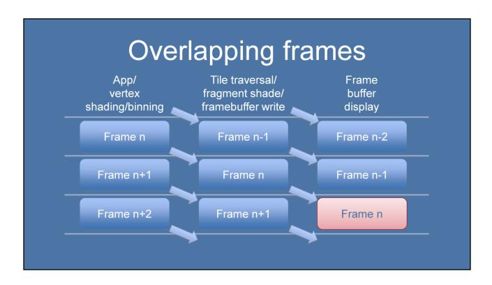
With this approach we end up implicitly triple-buffering – increasing throughput, but with multi-frame latency.
