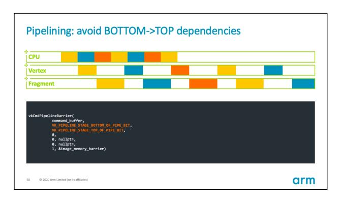
In GPUs like Mali we find two processing slots to do vertex and fragment work in parallel.
