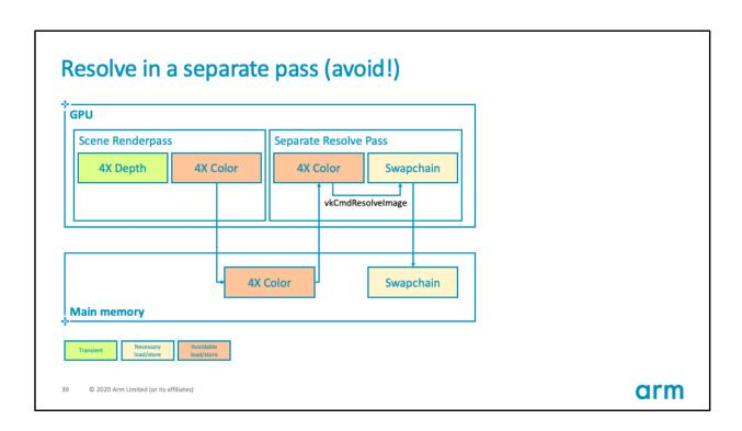
In contrast, if you use vkCmdResolveImage, the GPU will need to store the large multisampled attachment to main memory, and then read it back in a separate pass to resolve it, which is unnecessarily making use of a great deal of bandwidth and power.
