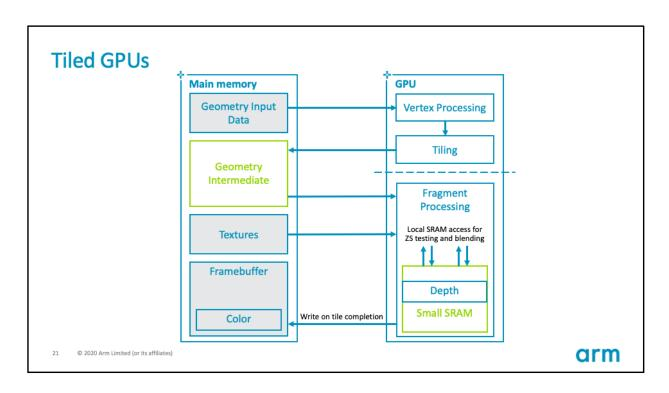
Therefore, depth does not need to be allocated at all in main memory, it can simply live temporarily in tile-local memory.
