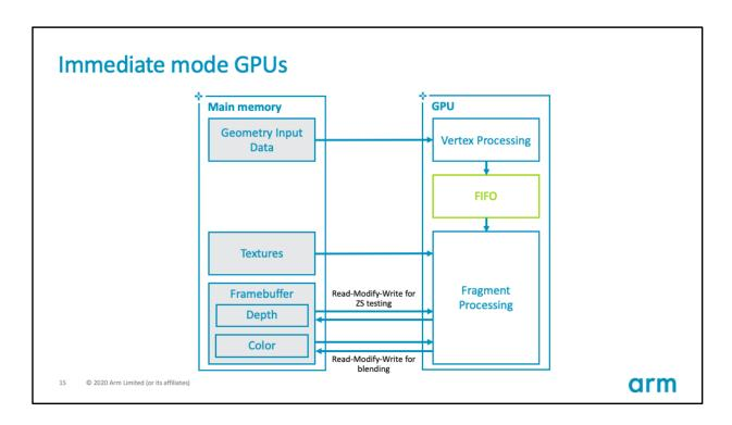
The GPU needs to load and store data to main memory, and here we represent these operations with arrows.
