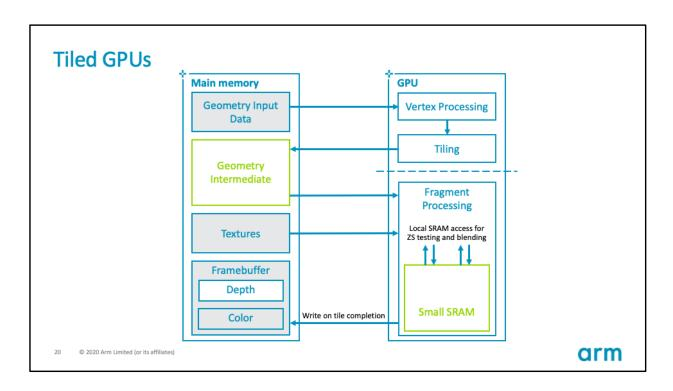
If we go back to our tile-rendering diagram, you can see that we can perform depth testing using tile local memory.
