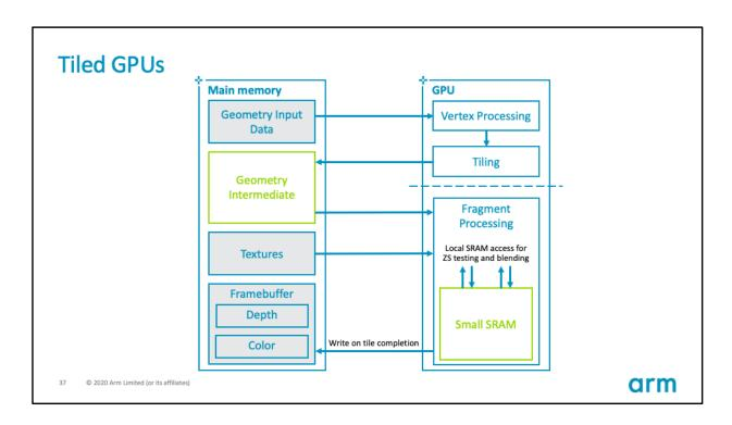
If we carry out this resolve operation in tile local memory, we do not need to write out the value of all the samples to main memory, and can therefore save bandwidth.
