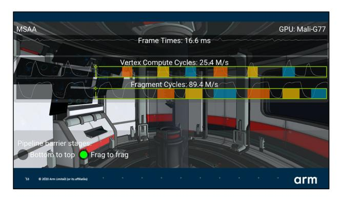
In the case of a fragment to fragment barrier, most of the vertex peaks occur in parallel to the fragment plateau, which is what we want.
