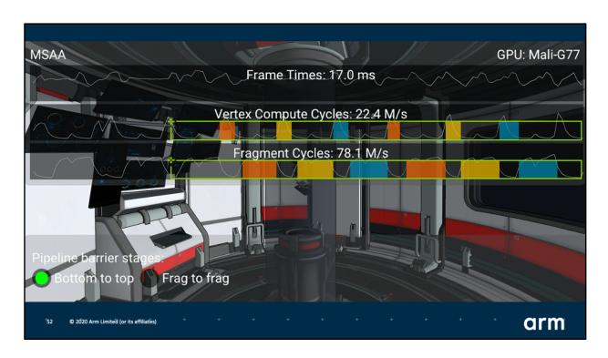
In the case of the MSAA sample this is how these bubbles can be visualized using the vertex and fragment cycle counters.
