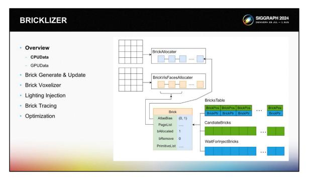
The core data structure in the CPU is illustrated as follows. During initialization, two allocators are initialized based on the given texture sizes of BrickMappingAtlas and BrickVisFacesAtlas, and an array is created by stringing together the Bias as the base elements. Some important parameters in Brick are:
