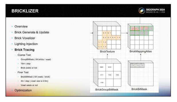
Utilizing BrickGroupBitMask and BrickBitMask, the HDDA algorithm can be implemented, enabling fast raycasting and intersection detection. The specific processing logic is as follows:
