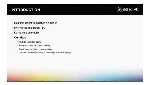
With a considerable amount of learning and struggling, we finally reached the point that a brand new voxel-based algorithm is coming up. It was built on the efficient sparse octrees and cache-friendly clipmaps to achieving a multi-level voxel-based scene representation.
