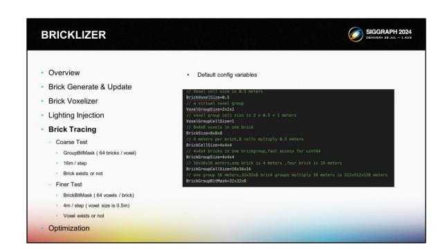
Here are the default config variables. The default voxelsize is 0.5 meters, there are 8x8x8 voxels in one brick, thus one brick covers the range of 4 meters. There are 4x4x4 bricks in one brickgroup, so the brickgroup covers the range of 16 meters. We have the number of 32x32x8 brickgroups , so the we can cover 512x512x128 meters.
